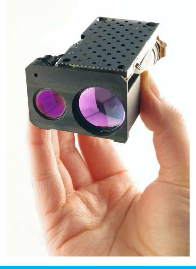
The compact, eye safe and highly integrated LRX laser rangefinder is utilized in various applications, from demanding military measurements to handheld devices.
